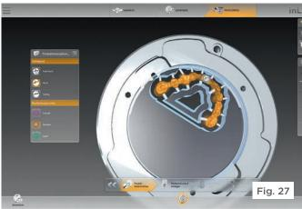
For the production, the resulting job was transferred to the inLab CAM SW 16.0 (Fig. 25), where the restoration, the sprues, and the sinter support, required for the subsequent sintering process (Fig. 26) were positioned and the milling job initiated (Fig. 27).
