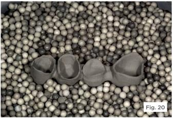
Since the inCoris CCB blank is made of a sintering metal, the next step was the sintering step that brought the framework to its final size and strength (Fig. 20). This step was performed in the inFire HTC speed sintering furnace (Dentsply Sirona CAD/CAM). For NPM sintering, the furnace is fitted with an argon gas connection and a separate sintering platform.
