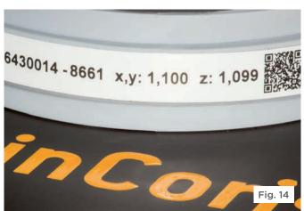
In the current version of the CAM software, the inCoris CCB blank can easily be identified by QR code detected by a webcam (Fig. 14) — a convenient feature that can also be used for all other inCoris blanks. The QR code provides all of the necessary information on the current blank without the inconvenience of manual data entry; the software even recognizes already partially milled blanks.
