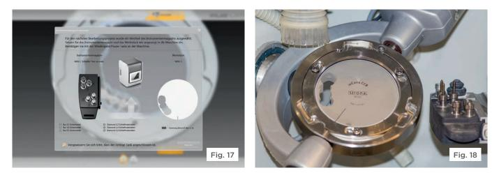
The software presents a reminder screen at this point (Fig. 17) to ensure that both the correct workpiece and the corresponding tool magazine are loaded into the unit (Fig. 18).
