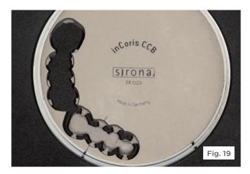
After 20 minutes of wet milling, the workpiece with the milled bridge framework is removed from the inLab MC X5 (Fig. 19). The blank was allowed to dry overnight and the framework separated the next day.
