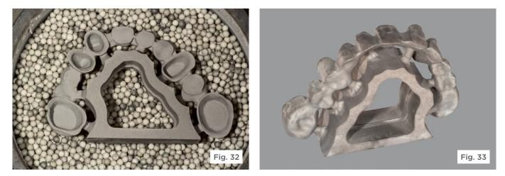
The final dimensions of the bridge framework were once again obtained by sintering in the inFire HTC speed (Figs. 32-33). Due to the large dimensions of the framework, sintering was performed with the aid of a sinter support – a procedure generally recommended for 6-unit and larger frameworks. The sintered framework was then veneered and finished.
