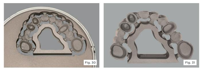
The bridge framework is then removed from the milling unit (Fig. 30) and separated for overnight drying (Fig. 31).
